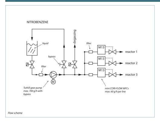
The new nitrobenzene dosing system comprises a Tuthill gear pump, a degassing valve, three M13 mini CORI-FLOW mass flow controllers with filters and some additional equipment. The degassing valve between the gear pump and the M13's is necessary to tackle the problem of gas bubbles in the nitrobenzene liquid.
